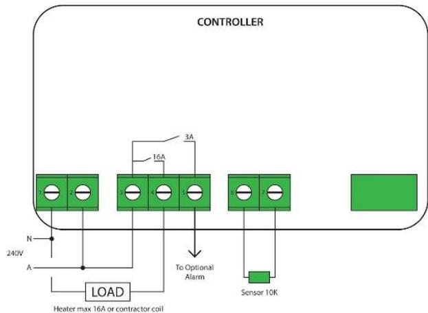
*Note: The sensor resistance is 10 k ohm at 25 DegC and 30 k ohm at 0 DegC*
